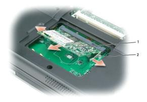
1 Mini PCI card 2 metal securing tabs (2)
